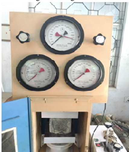
Fig.4. Testing of Cubes
