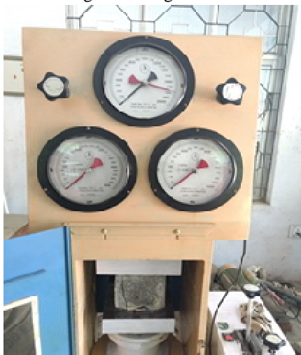
Fig.4. Testing of Cubes
