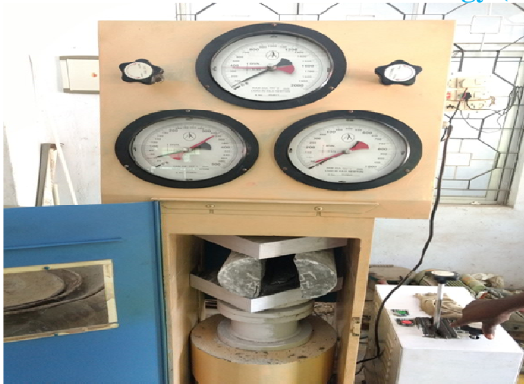
Fig.6. Testing of Cylinder for split tensile strength
