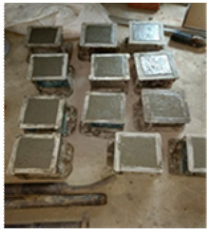
Fig.2. Casting of cubes
