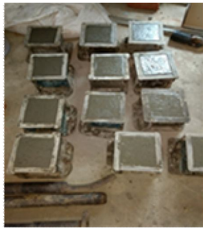
Fig.2. Casting of cubes
