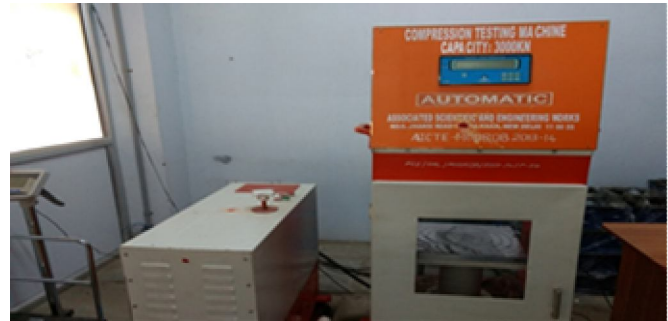
Fig.3. Automatic Compression Testing Machine
