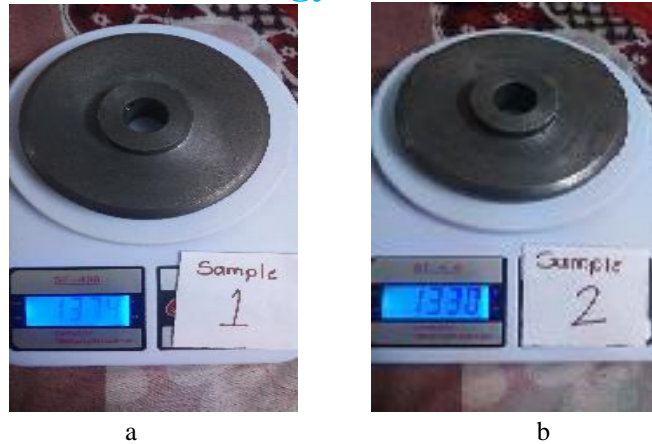
Fig. 1. Base material casing after machining a- sample 1, b- sample 2
