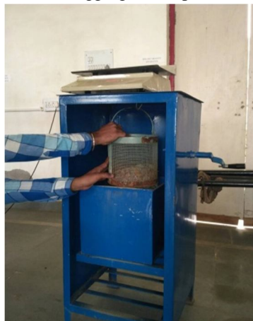
Fig. 3 Wire bucket for Specific gravity
