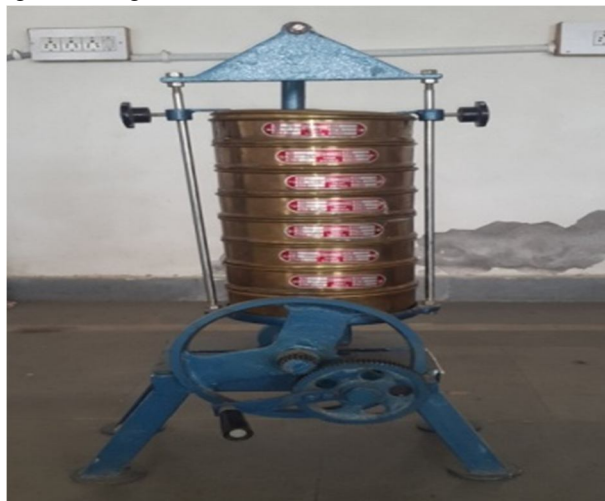
Fig 1 Sieve shaker with sets of sieve
