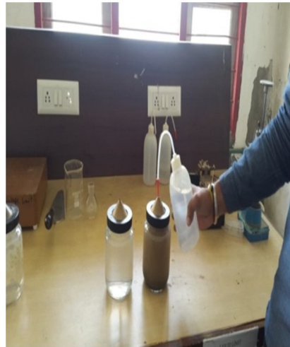
Fig 2 Pycnometer bottle for specific gravity
