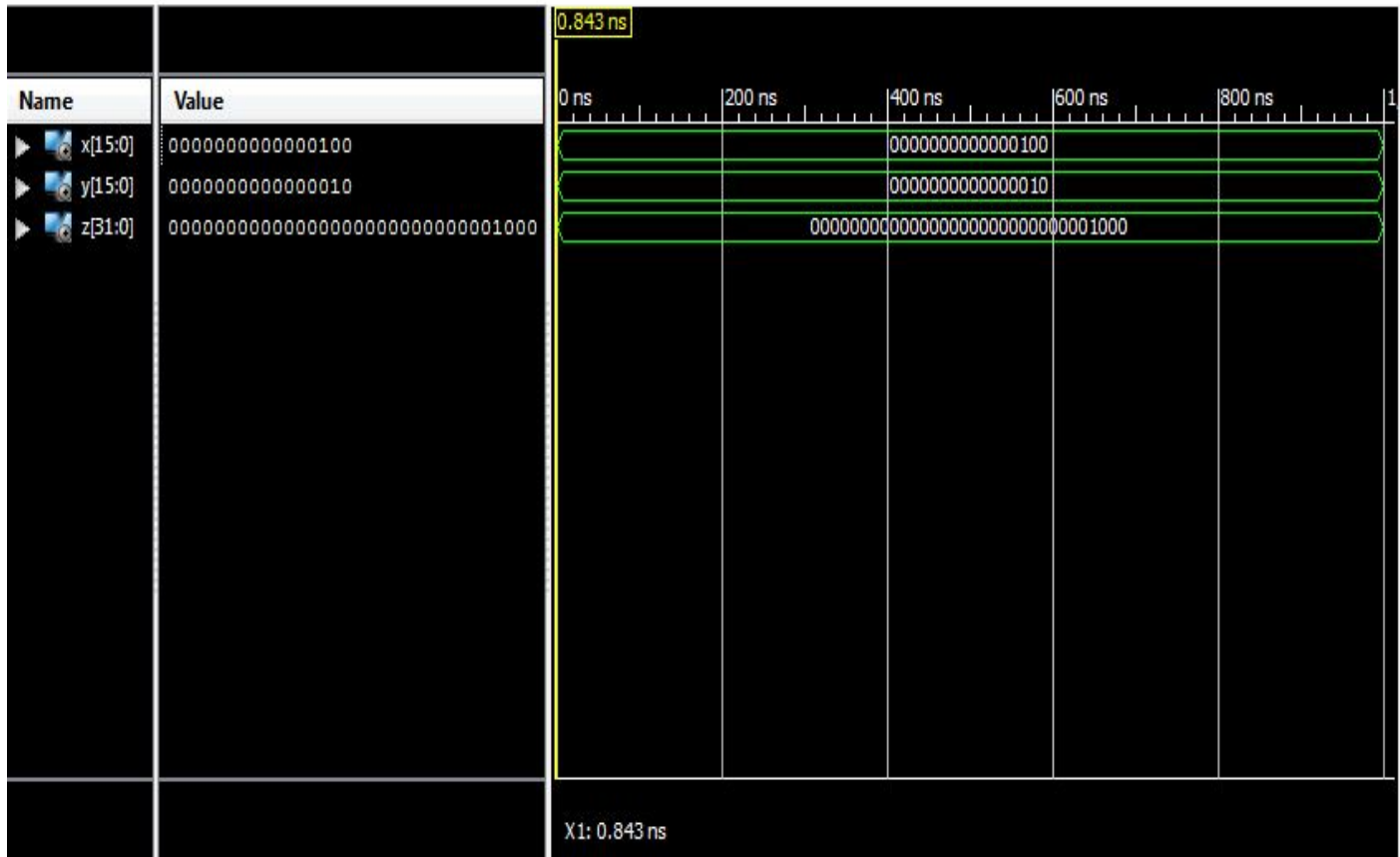
Fig-5:-simulation result of Vedic multiplier
