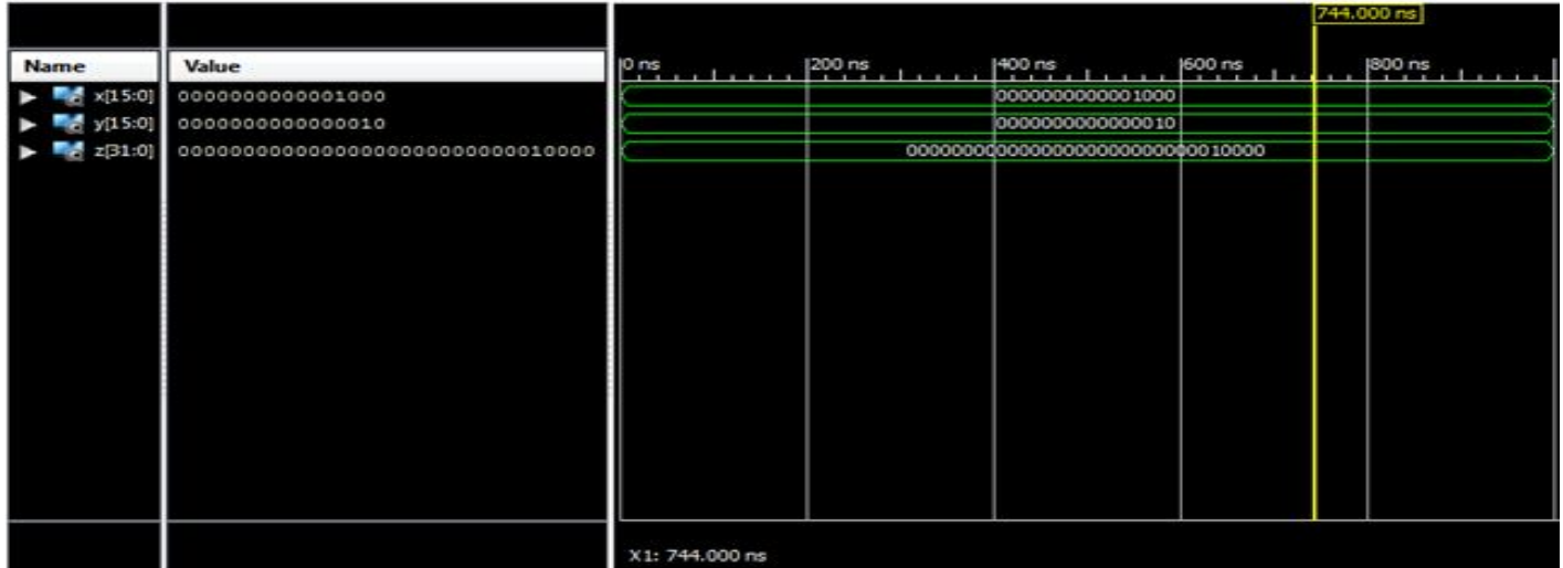
Fig-4:-simulation result of Booth multiplier
