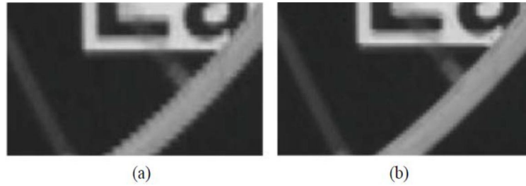
Figure 1. De-interlaced results: (a) linear versus (b) edge-adaptive algorithm.
