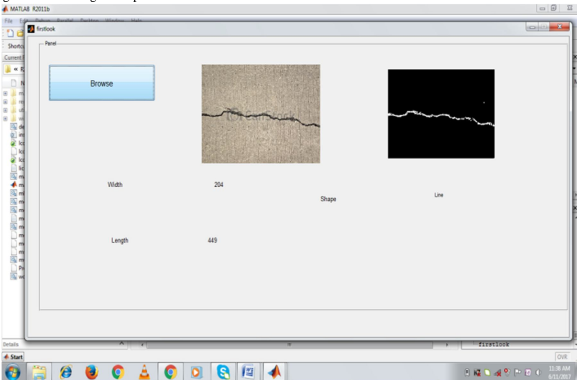
Fig. 5: Road Image with detected edge and parameters calculated on it.
