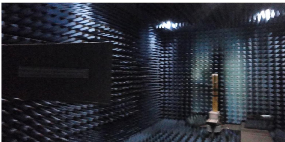
Figure 11 Measurement of radiation pattern for a Z-U-T-S shaped antenna in an anechoic chamber
