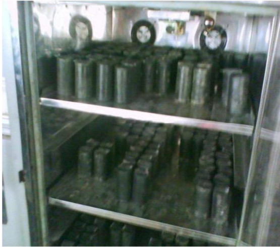
Fig: Lime stabilized fly ash coated with Wax
