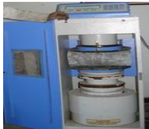
Fig.5 split tensile strength testing
