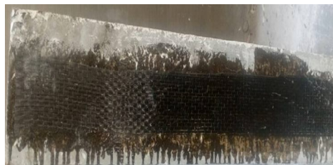
Figure 3 Half side wrapping
