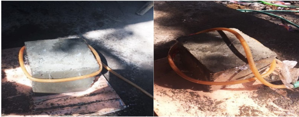
Figure no 3:- Curing of concrete block using drip curing
