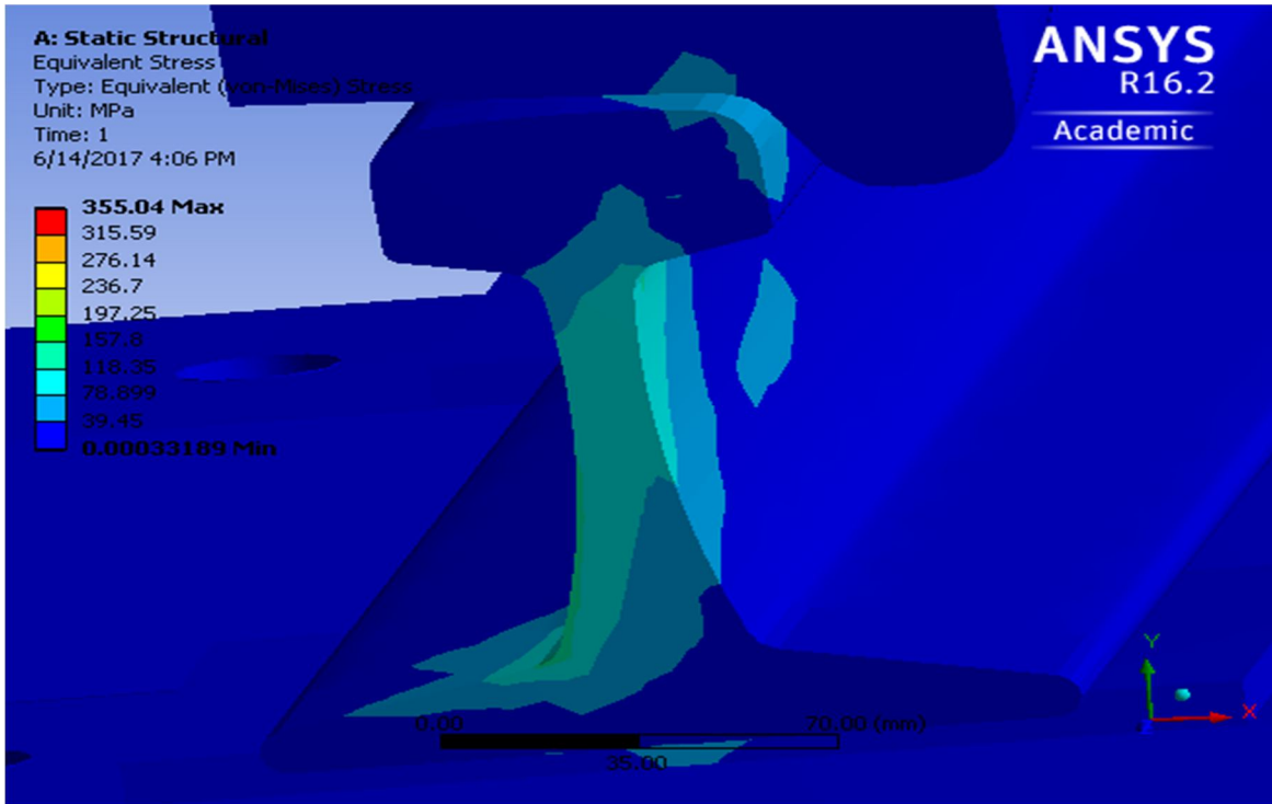
Fig8. Sectional view of Maximum Equivalent Von-Mises stress in left rail with 835m curvature.
