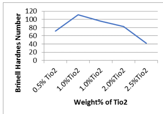
Figure 1.8: BHN Vs Weight% of TiO 2 curve.
