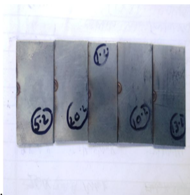
Figure 5 Vickers Microhardness test specimens
