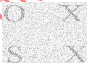
Fig. 13 Recovered encrypted watermark with SNR=40db
