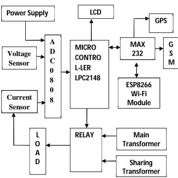
In this project uses regulated 12V, 500mA power supply. The 7805 three terminal voltage regulator is used for voltage regulation. Bridge type full wave rectifier is used to rectify the ac output of secondary of 230/12V step down transformer.
