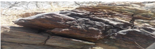
F. Gossan zone in sheared quartzite near old working of copper mining.
