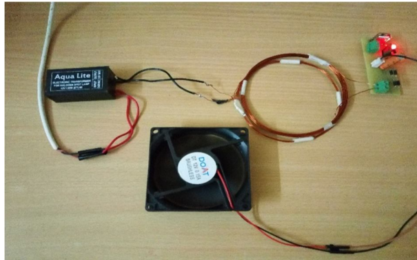
Fig. 3 Wireless Power Transfer for Fan
