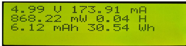
Fig. 5 (a) The Voltage and Current Display at the micro- controller side
