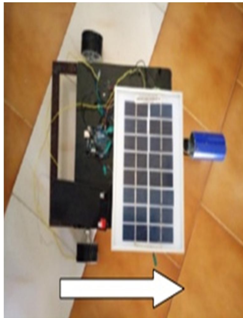
Fig 2: Vehicle turning towards right after sensing obstacle
