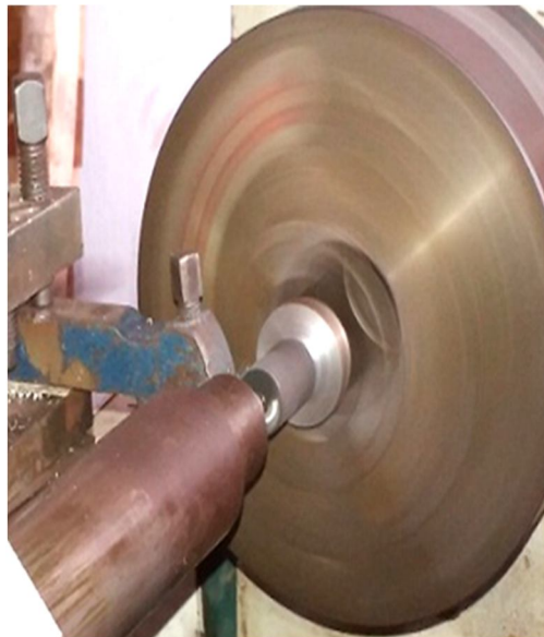
Fig 1: Sample preparation for machining performance test
