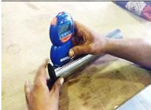
Figure 5 Surface Roughness Testing
