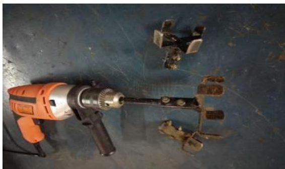
Power operated soil stirrer for home gardening
