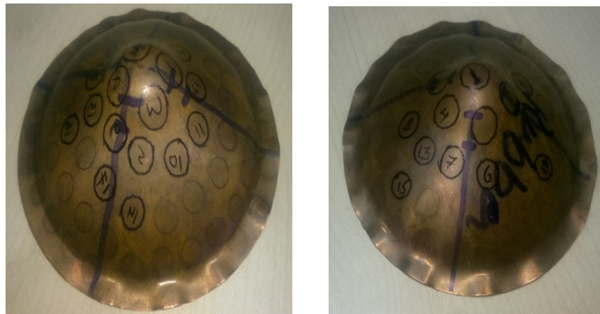
Figure 6: Sheet metal forming with rubber and without rubber in stage III
