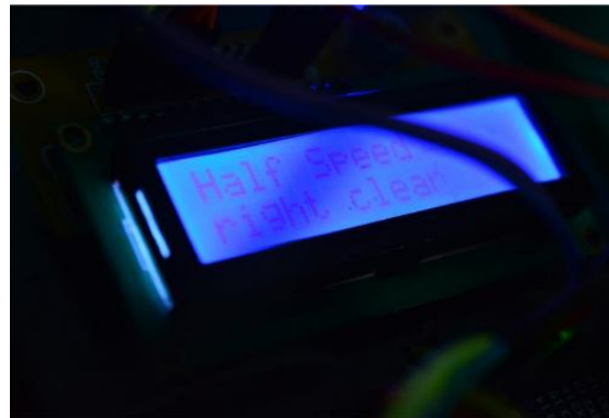
Fig 7: when the vehicle is detected at 20 cm, Right clear
