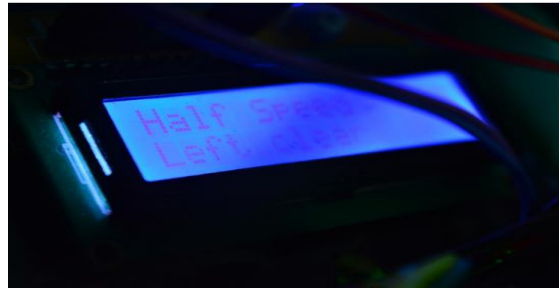
Fig 6: when the vehicle is detected at 20 cm, Left clear
