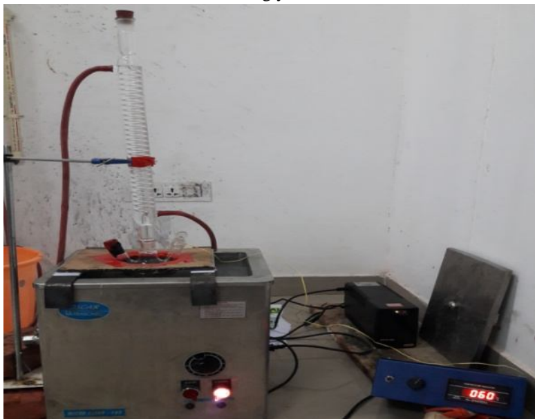
Fig. 1 Ultrasonicator Set-up for Biodiesel Production with Condenser and Digital Thermocouple
