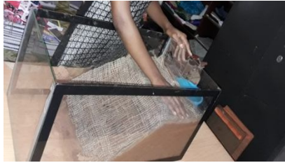
Fig 10: Jute Geo Textile on the compacted soil slope
