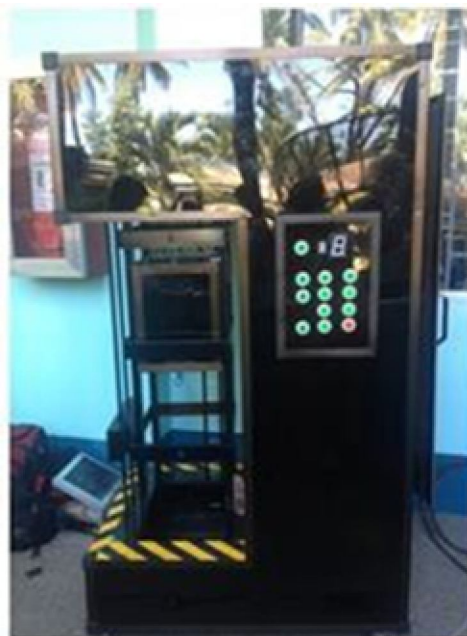
Figure 4 Completed prototype of the Three-lift Elevator Instructional Device
