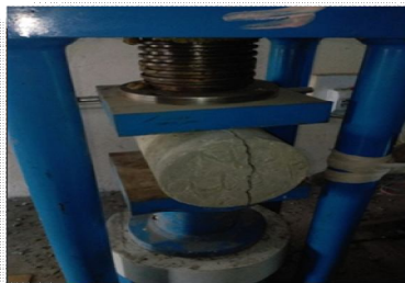
Fig 3: Shows Split Tensile Strength Test of cylinder
