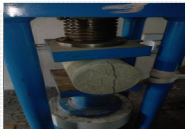
Fig 3: Shows Split Tensile Strength Test of cylinder
