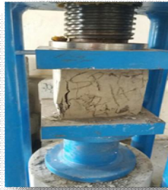
Fig 2: Shows Compressive Strength Test of Cube
