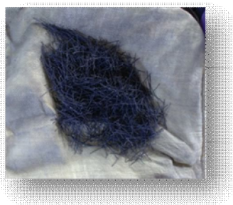
Fig no 1: Shows Plain Steel Fibres Are Discrete To Distribute Uniformly In the Concrete Mix
