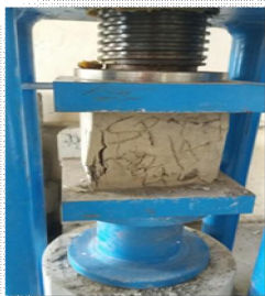
Fig 2: Shows Compressive Strength Test of Cube
