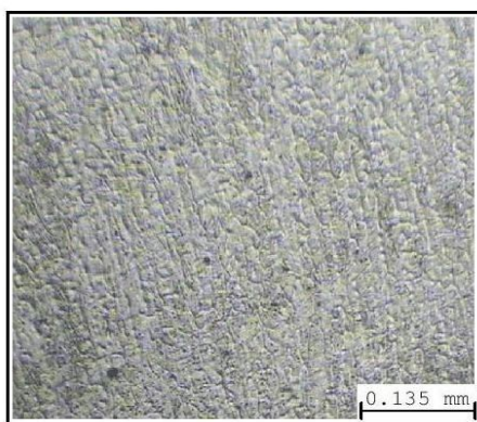
Fig. 10 Microstructure for E410 electrode weld metal
