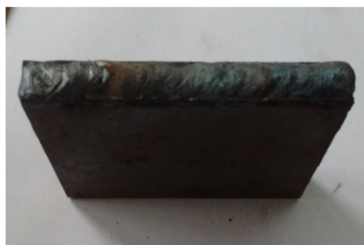
Fig. 2 Deposition of weld metal on base metal
