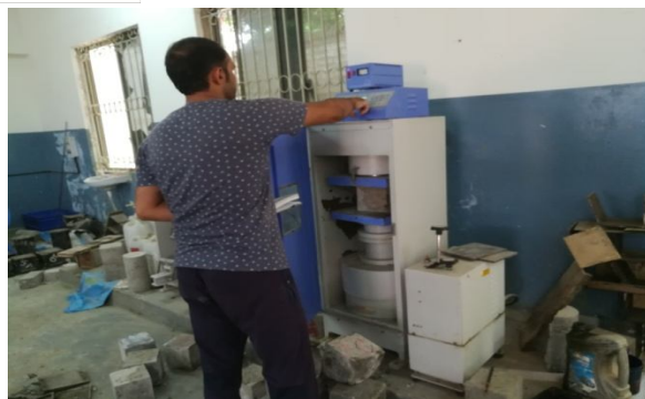
figure:4.compressive strength test of cubes.
