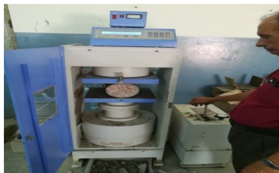
figure:5.Split Tensile strength of cylinders
