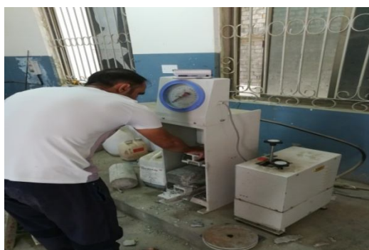
Figure:6. Flexural strength test of beam
