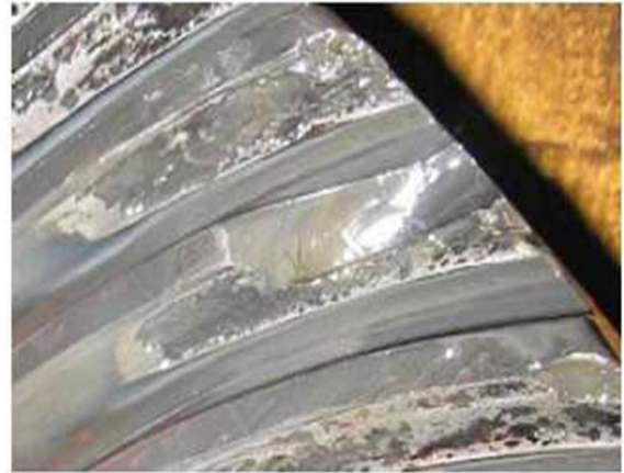
Figure 2: beach marks on gear
