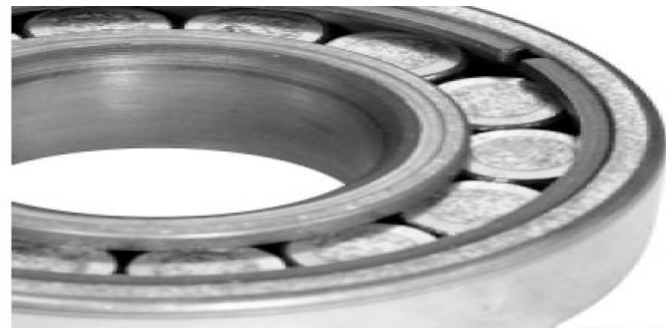
fig 6: Etching on roller bearing
