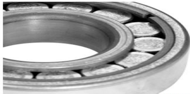
fig 6: Etching on roller bearing
