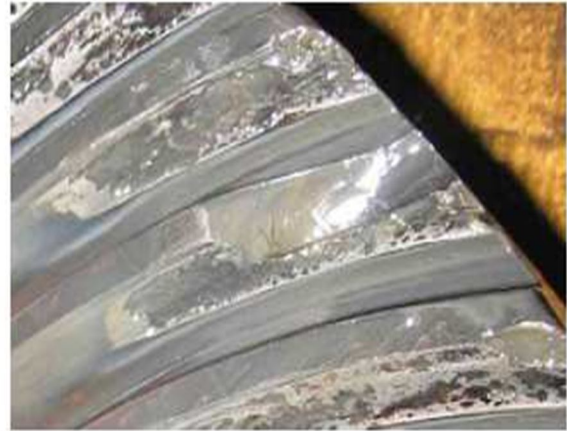
Figure 2: beach marks on gear
