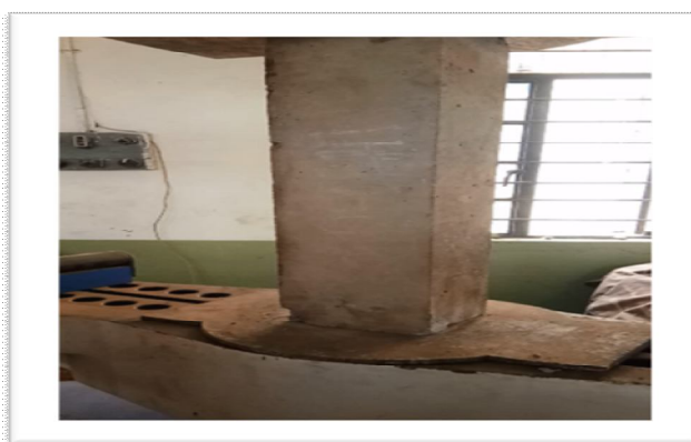
b) 700 mm column specimen tested on UTM
