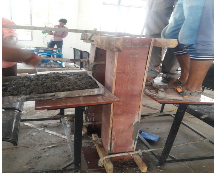
Figure 4: Mixing and Casting of RC Column Specimen
