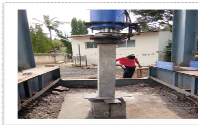
a) 1100 column specimen tested on Hydraulic loading frame
