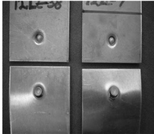
2.8 Representative image of SPR joint assemblies exhibiting rivet tail pullout. Images shown are lap shear coupon assemblies after testing.
