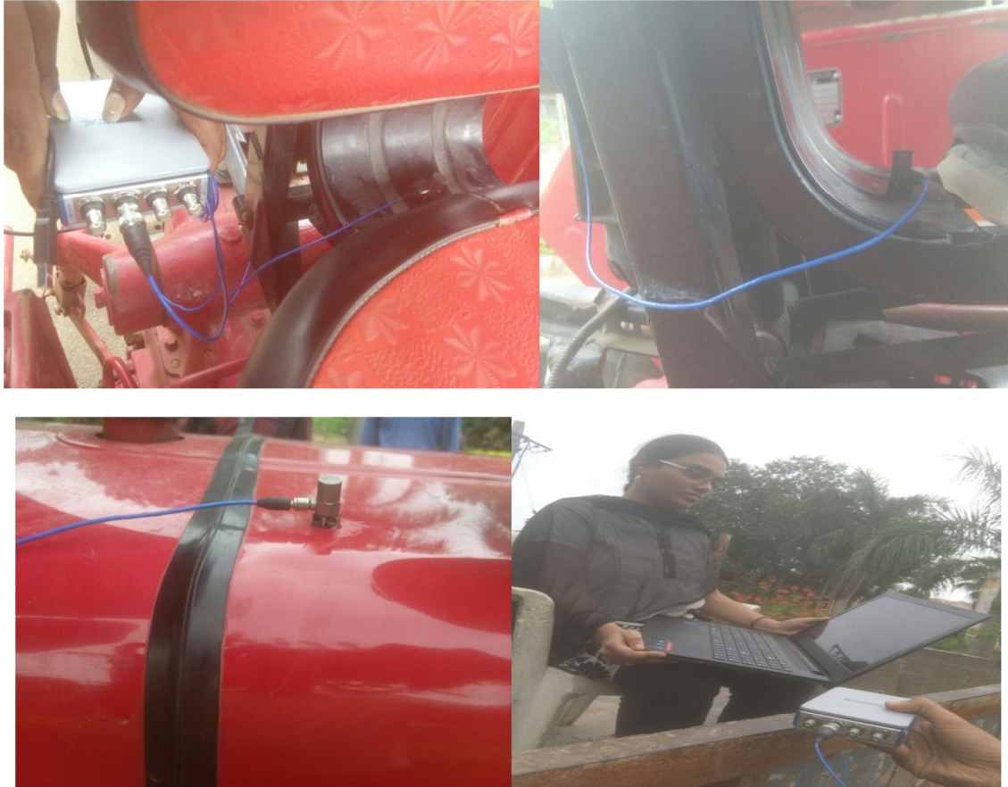
Fig.4 Experimental analysis of tractor seat frame and tractor bonnet by using FFT analyzer
