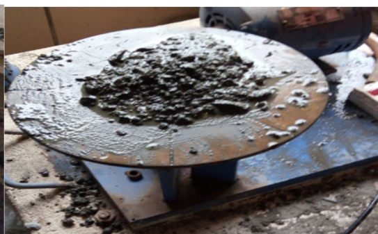
Fig 3.2 Flow table test.
