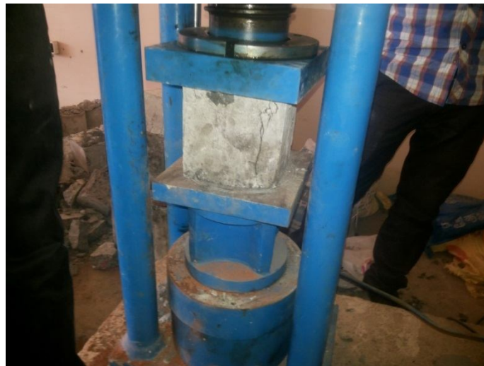
Fig. 3.3. Compressive Strength Test.
