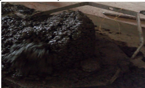
Fig 3.1 Slump cone test.
