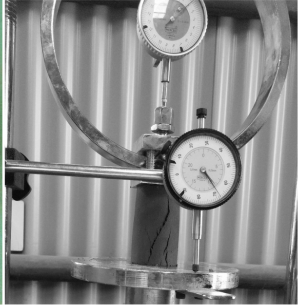
Fig. 2. Soil Sample under Unconfined Compression Testing Machine showing start of failure.
