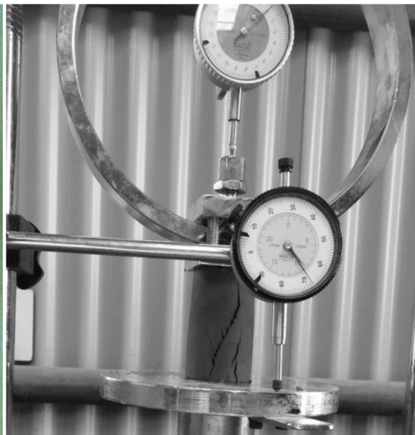
Fig. 2. Soil Sample under Unconfined Compression Testing Machine showing start of failure.
