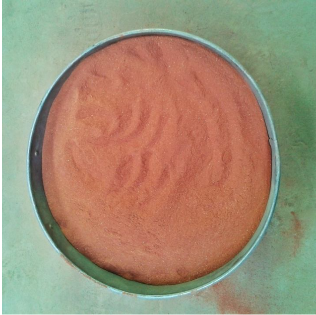
Fig.1.2 Waste brick powder after being sieved through 1.1mm IS Sieve.
