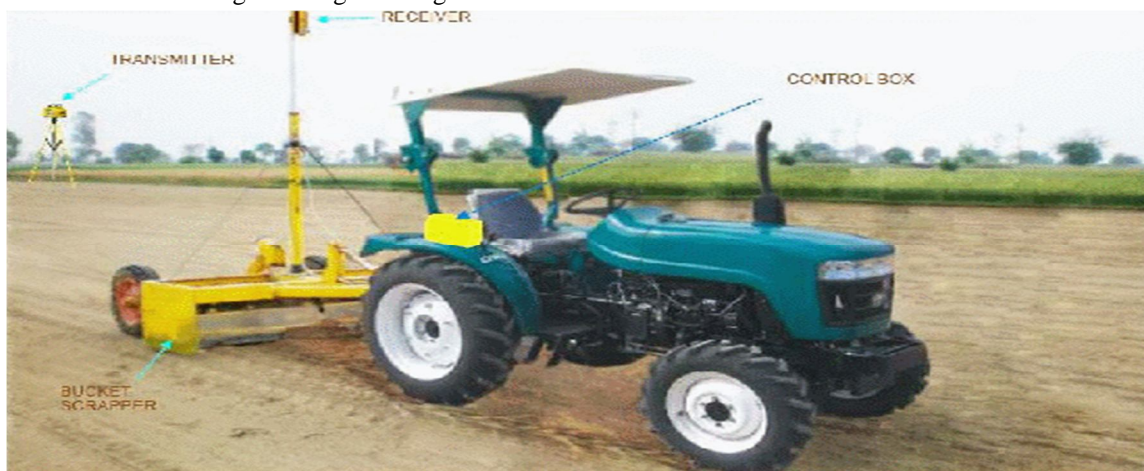
Figure 1: Settlement of Lands System Using Laser Technology
