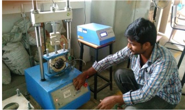
Fig.6: Marshall Stability Test Equipment
