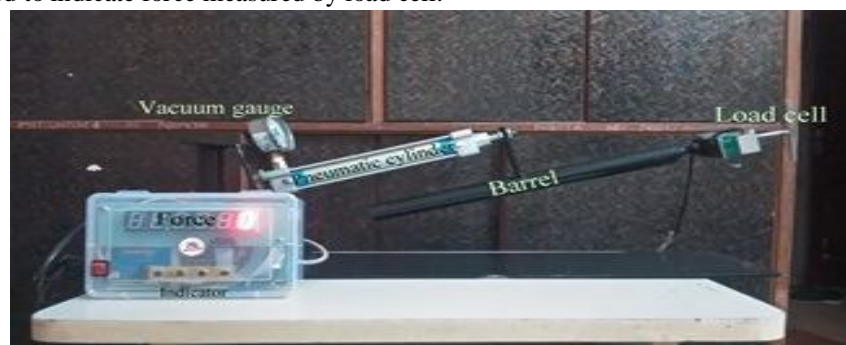
Fig. 1 Experimental Model of vacuum damped recoil system
