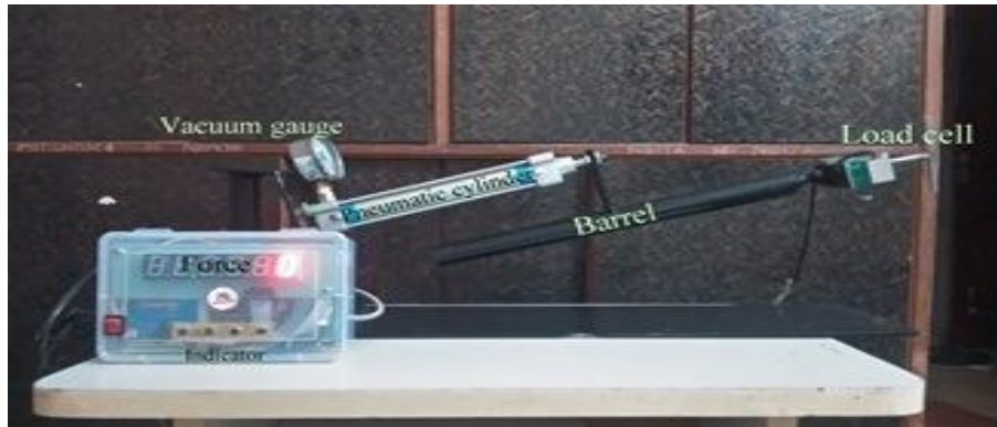
Fig. 1 Experimental Model of vacuum damped recoil system
