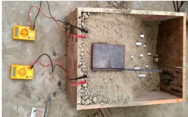
Fig.7 Soil nailed slope before loading
