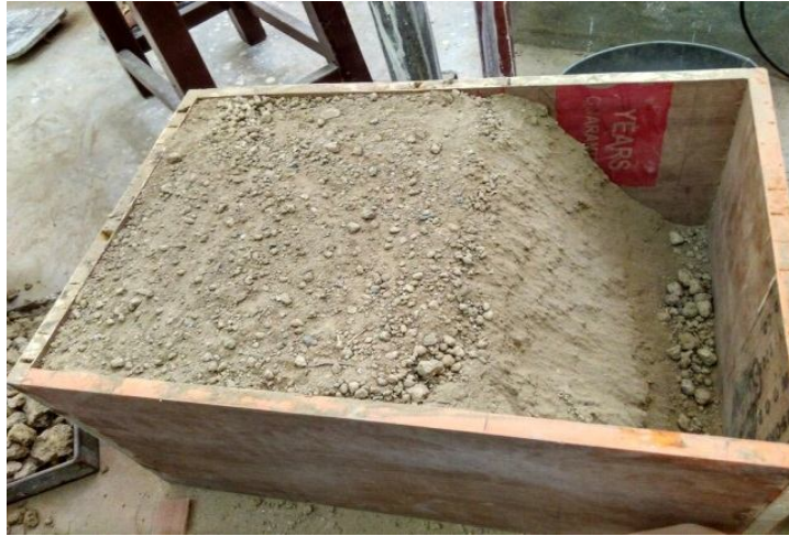
Fig.5 Unreinforced soil slope( 60^\circ )
