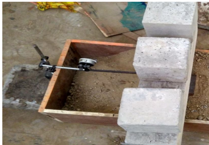
Fig.8 Loading on unreinforced soil slope.
