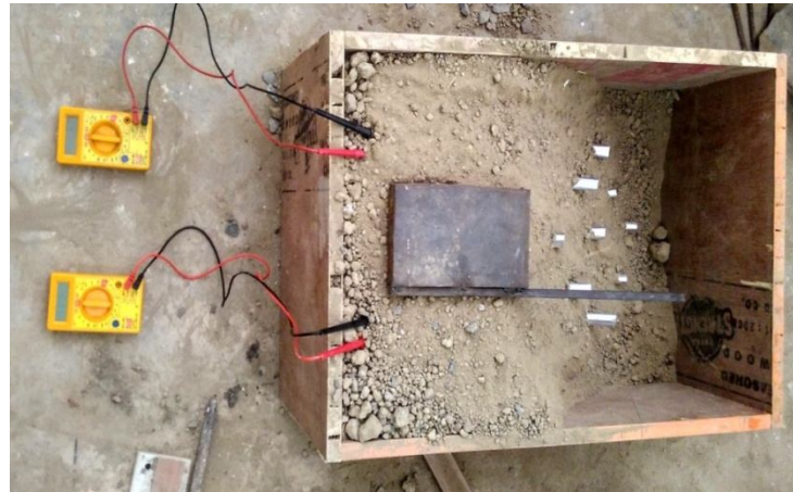
Fig.7 Soil nailed slope before loading
