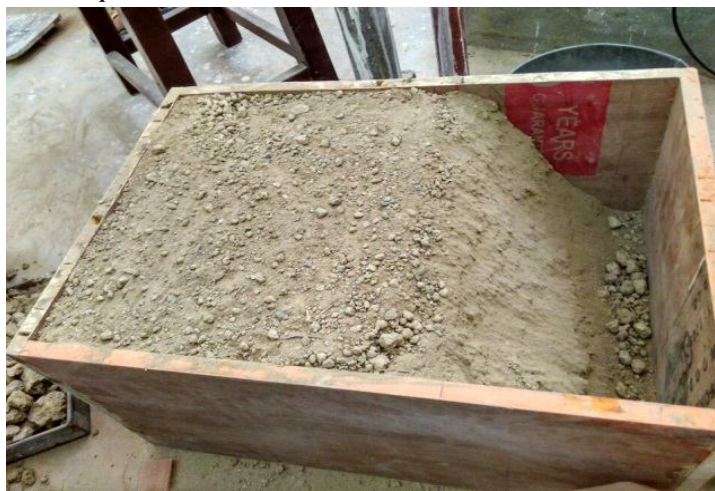
Fig.5 Unreinforced soil slope( 60^\circ )
