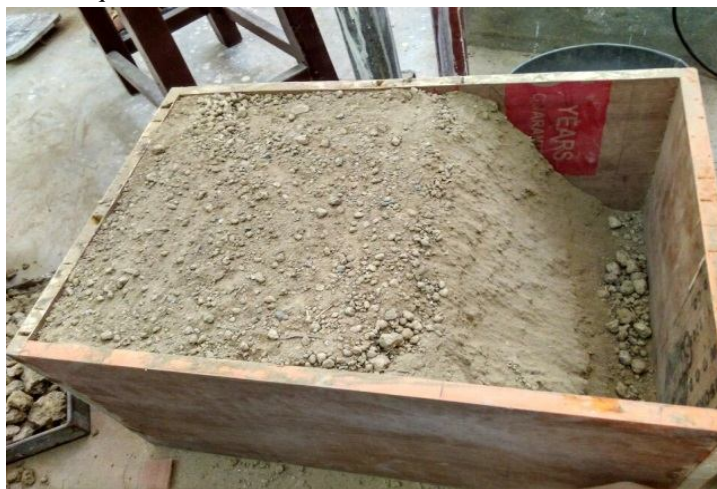
Fig.5 Unreinforced soil slope( 60^\circ )
