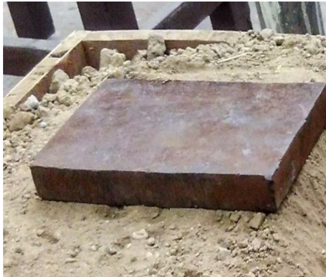
Fig. 4 Mild Steel Bearing Plate
