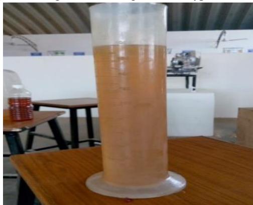
Fig.2. Blending diesel with mahua biodiesel.
