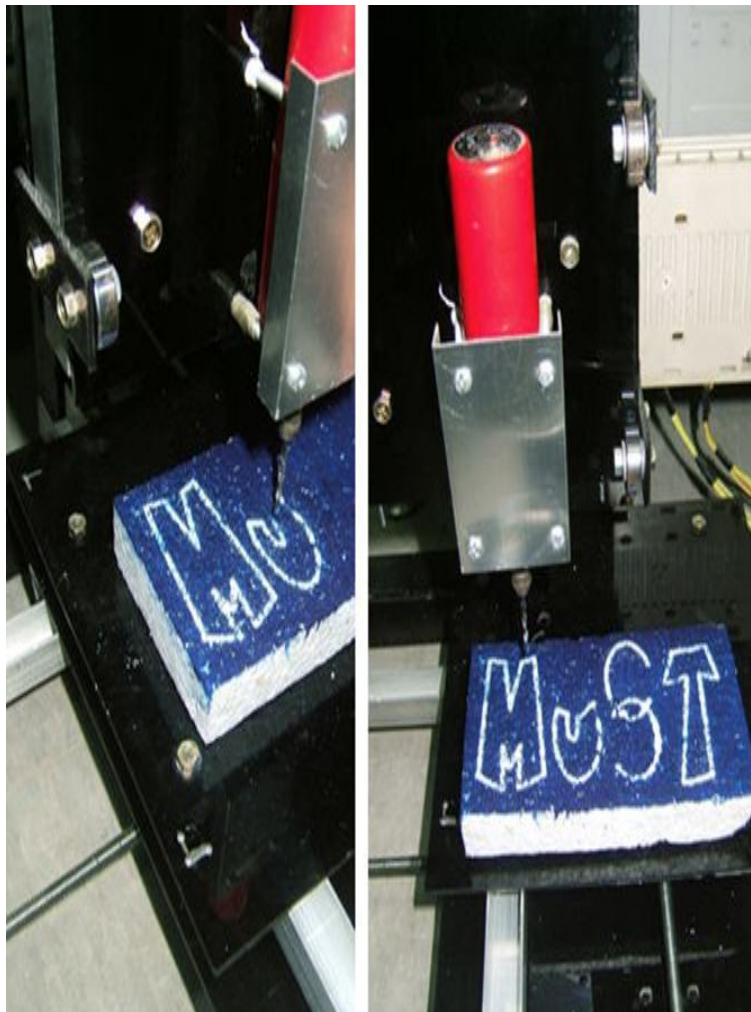
Figure 20: The milling operation
