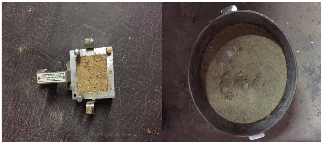
Figure 2 – Direct Shear Box with Mixed Specimen, CBR Test Mix Composition in Mould
