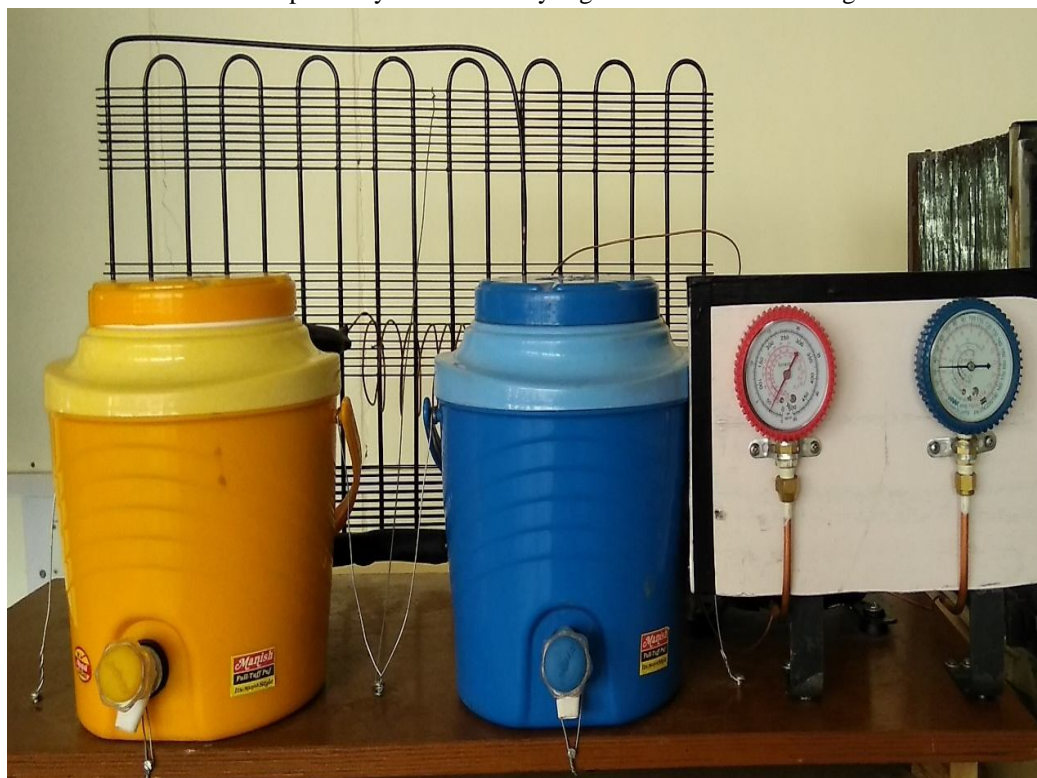
Fig. 2 Working VCERS working model (Front view)
