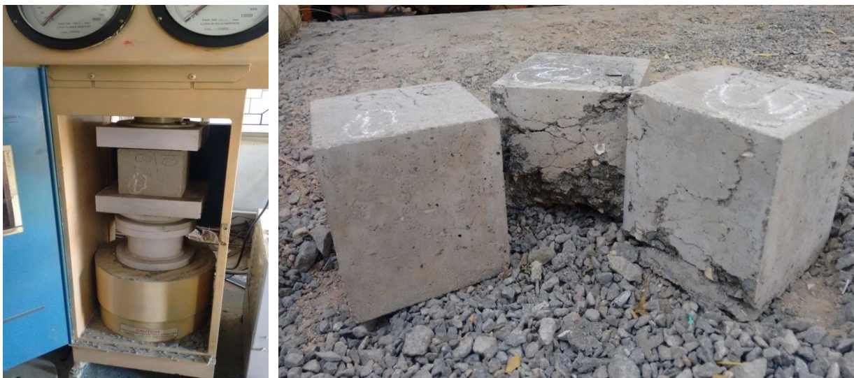
Fig.2. Compressive strength Test
