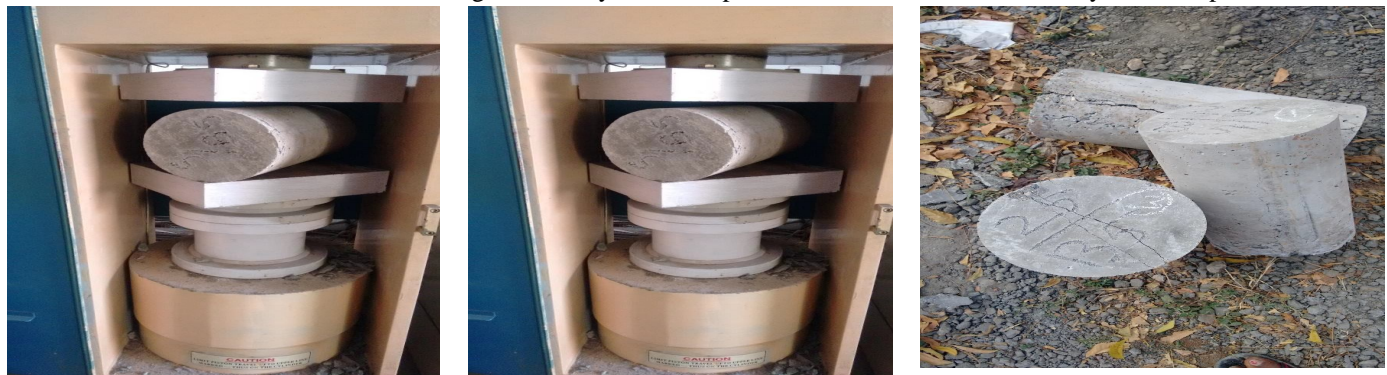
Fig.5. Split tensile strength test
