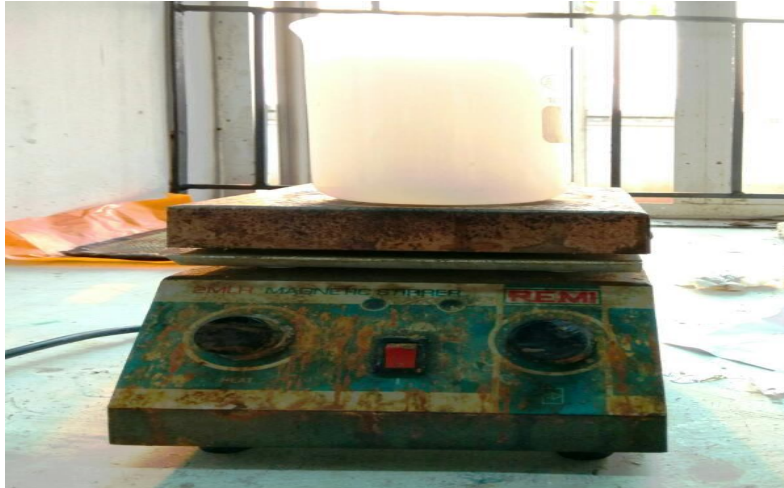
Fig.1: magnetic stirring of Al_2O_3 - H_2O
