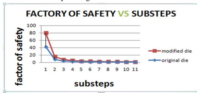
Graph-1: Graph shows Comparison of Factor of safety of Original die and Modified die
