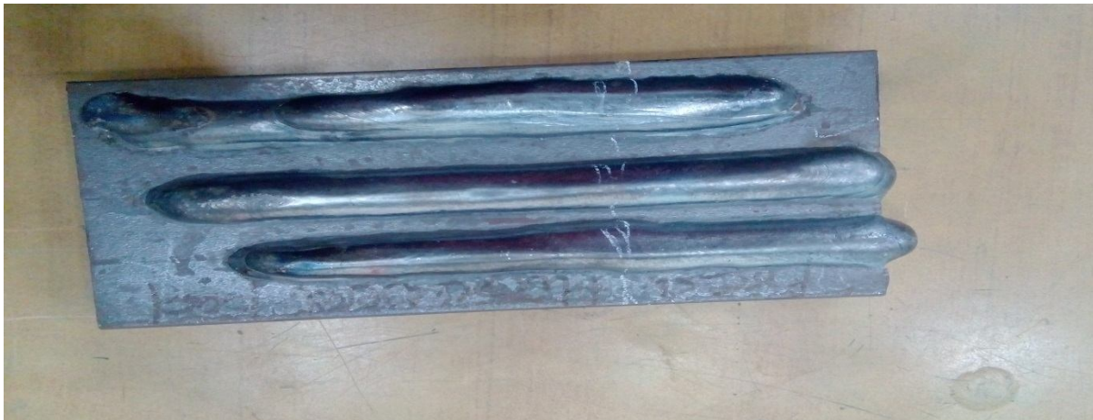
Fig:3 Fresh flux weld bead
