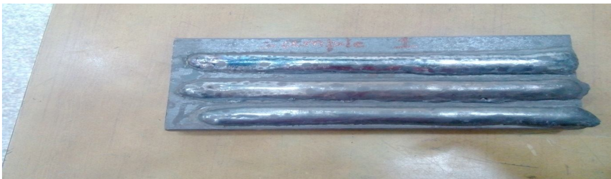
Fig 4: Recycled slag bead
