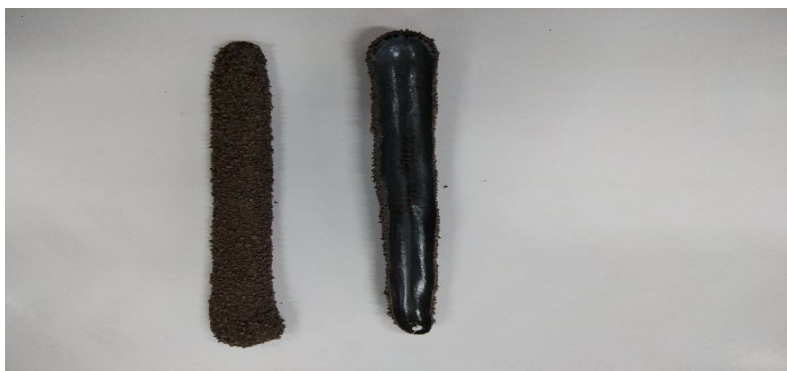
Fig:5 Slag Envelope after welding
