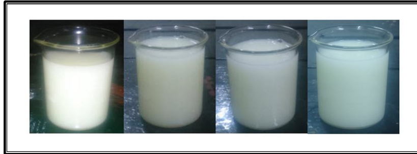
Fig. 1 showing emulsions made by mixing different ratio of water, diesel and surfactant K3 K2
